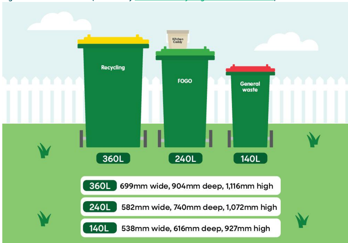
Figure 3.1: Bin Dimensions (Source: City Waste and Recycling Services information )
