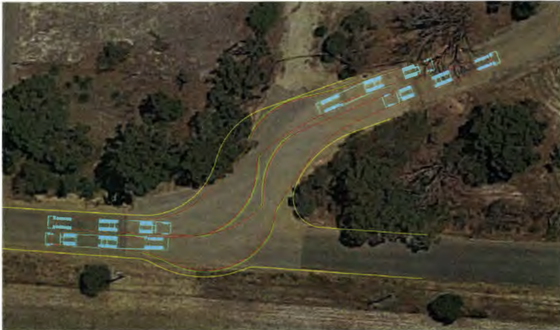
Figure 11 – Recommended Crossover Geometry
