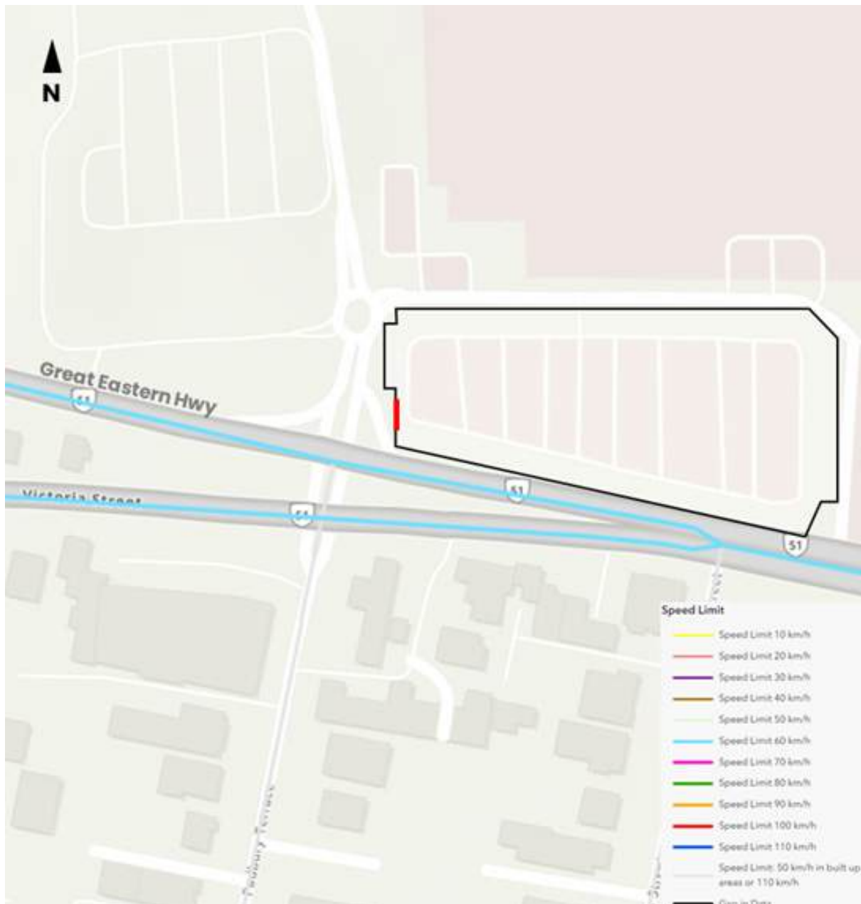
Figure 5 – Speed Limits on the Surrounding Road Network
